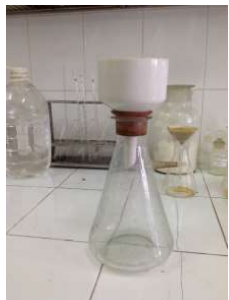
Washing the Sodium Hypochlorite from the oxidized starch
