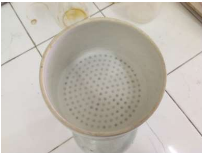
Washing the Sodium Hypochlorite from the oxidized starch
